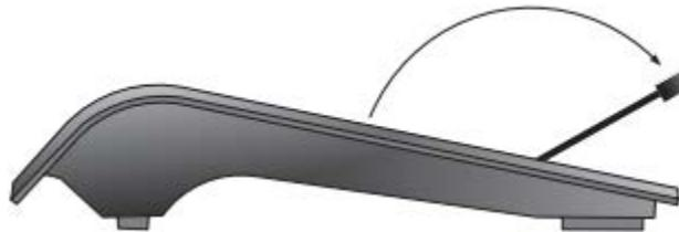
Figure 1-1: Flip out the Kickstand
